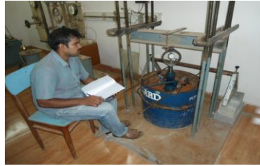
Author Conducting Static Plate Load Test
